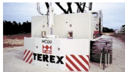
Hydraulic removable counterweight system
