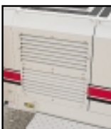
Main hydraulic system has separate cooler, hydraulically-driven fan. Cooler hydraulics — easier to maintain, longer lasting
