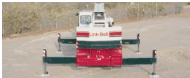
Fully Extended Outriggers 20' 6" (6.25 m) Spread
