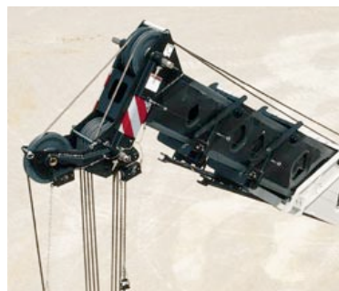
Basic boom extend mode – boom mode 'B'
