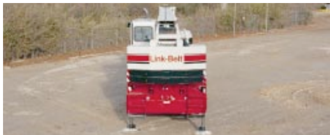
Retracted Outriggers 7' 9" (2.36 m) Spread
