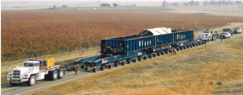
Bigge configured this 340 foot, 26 axle beam and dolly transporter to haul a 520 ton electrical generator.
