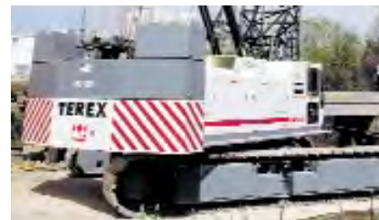
Counterweight hydraulically extends
