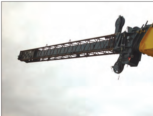
Max. tip height of 154 ft. (47.0 m) w/45 ft. (13.7 m) telescopic extension.
